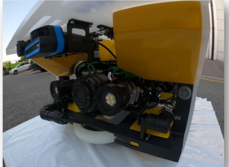
Demre ROV Front Camera and LED System with Tilt Capability
